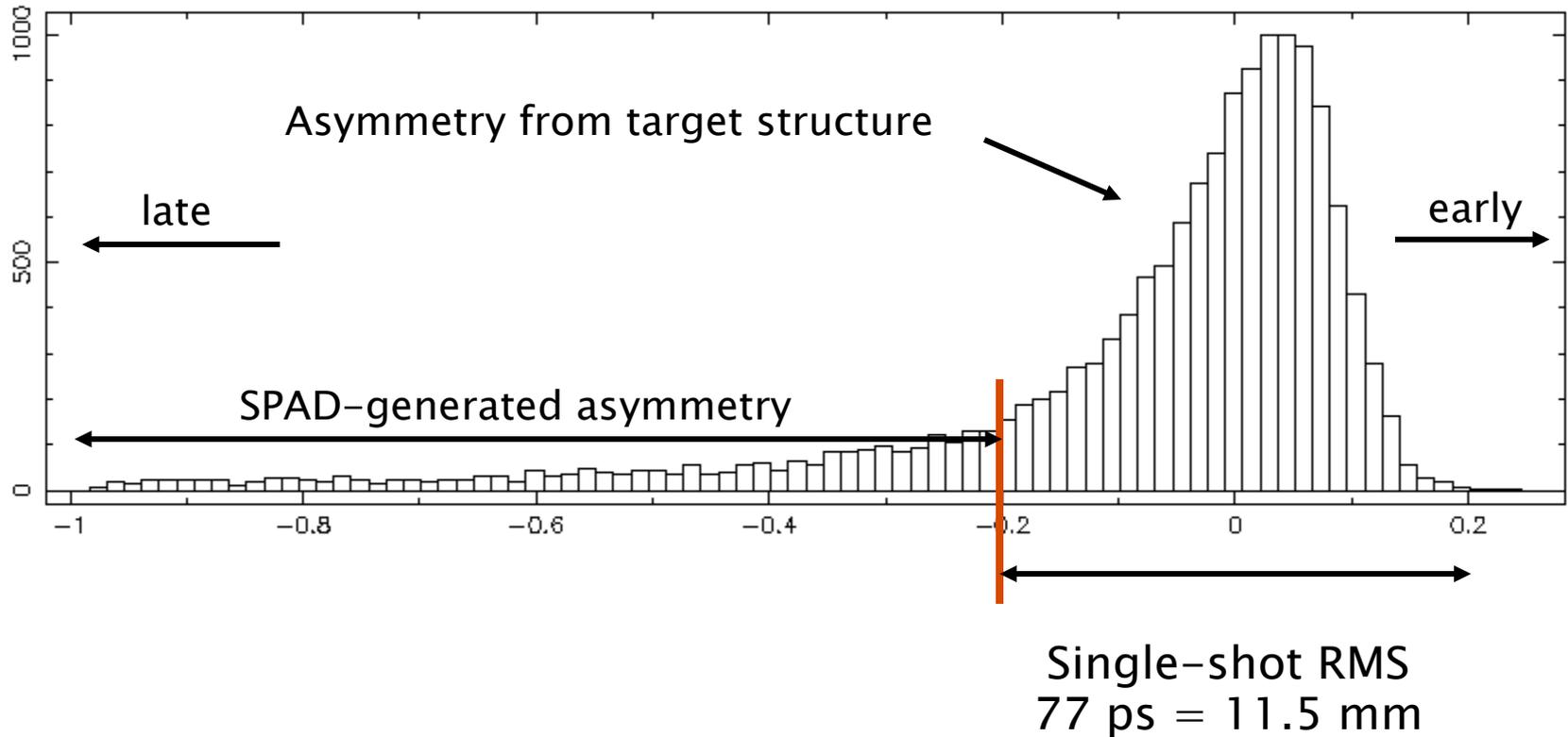
Target signature (retroreflectors at different target depths) plus SPAD asymmetric behaviour
